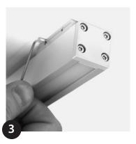
Secure slider to plate with hex key.
